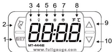
Figura 6: Controlador Digital MT 444E FASTON
