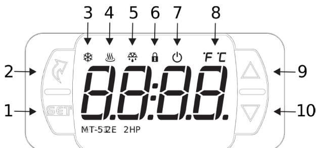
Figura 6: termostato MT-512E
