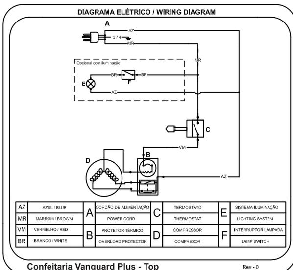
DIAGRAMA ELÉTRICO / WIRING DIAGRAM
